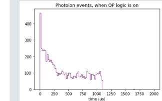
More atoms are photoionized when the polarization is low rather than when the polarization is high. Therefore we see a peak of ions at the start of a cycle and then see a drop later on. The ratio between the tail and the peak is used to estimate the polarization.
