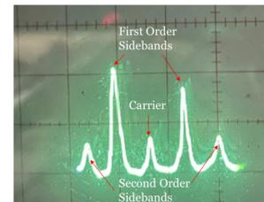
Used a scanning Fabray-Perot Interferometer to view frequencies and viewed on oscilloscope. For both the first and second order, the sidebands are asymmetrical, likely due to AM modulation superimposed on the FM modulation (cite paper). We average them to remove the AM component when doing the fit below.
