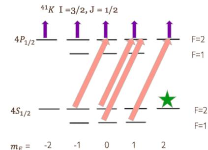
The atoms in the MOT are polarized by using optical pumping to move the atoms into the fully-stretched state. A 770nm circularly polarized laser is used so each cycle the excited atoms will be pushed one hyperfine splitting to right (for right circularly polarized light). The atoms then decay back down to the F=1 or F=2 state, and the process continues until the atom is stuck in the F = 2, mF = +2 state, called the fully-stretched state.
