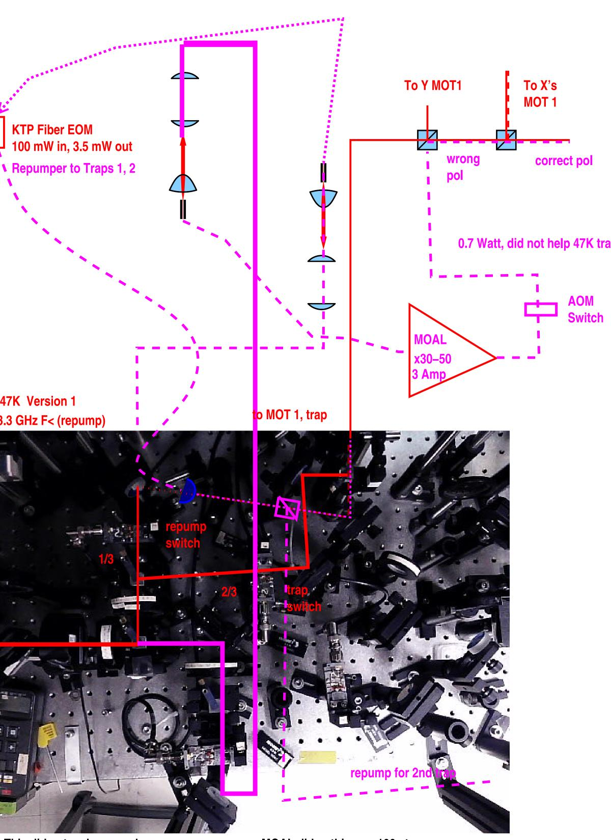
This did not make enough repumper power: e.g. MOAL did nothing –> 100 atoms So we moved repumper EOM fiber to MOAL and left it on all the time We also left OB light on all the time to be a repumper for 2nd trap
