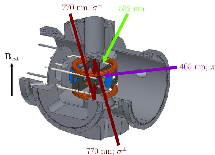
Fig. 3: Laser beams inside the MOT chamber. The optical pumping light enters the trap at an angle and is aligned by two very thin pellicle mirrors (70 nm Au on 4  $\mu\text{m}$  capton). Note that the probe light enters the trap from the side in order to preserve the  $\pi$ -polarization with respect to the quantization axis formed by the optical pumping light beams.
