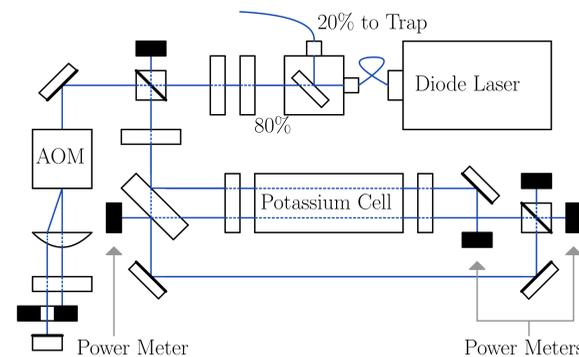
Fig. 2: Schematic of doppler free saturation absorption spectroscopy setup used to lock the 405 nm laser. The two power meters on the right are used to subtract the doppler broadened gaussian from the saturated signal. Instead of dithering the AOM or the laser we Zeeman dither the potassium cell using a coil around it (not shown here).
