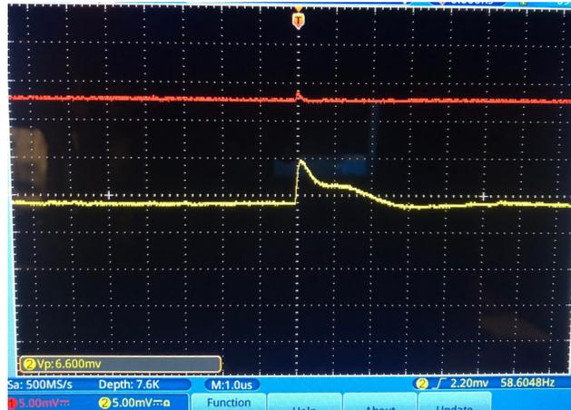
Figure 8: Raw timing (red) and energy (yellow) signal pulses.
