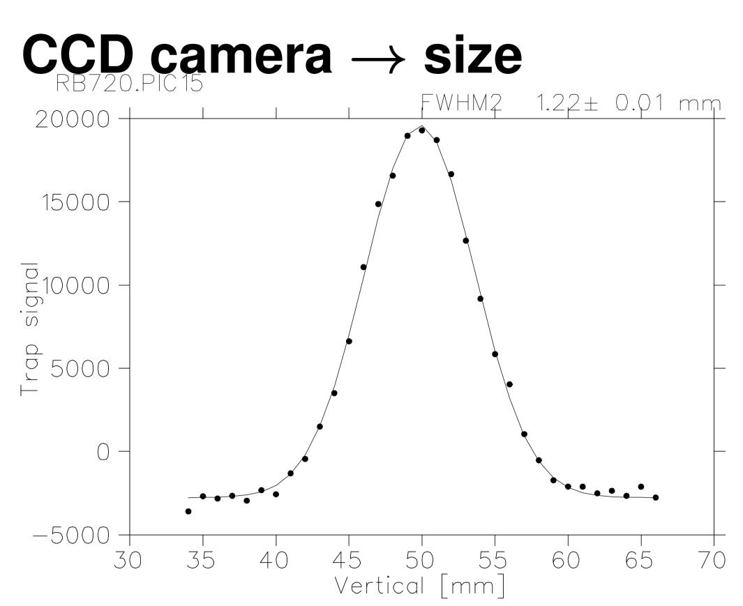
So settled for our main goal, minimizing the cloud size in a simple CCD camera with 200 millsec exposures:
