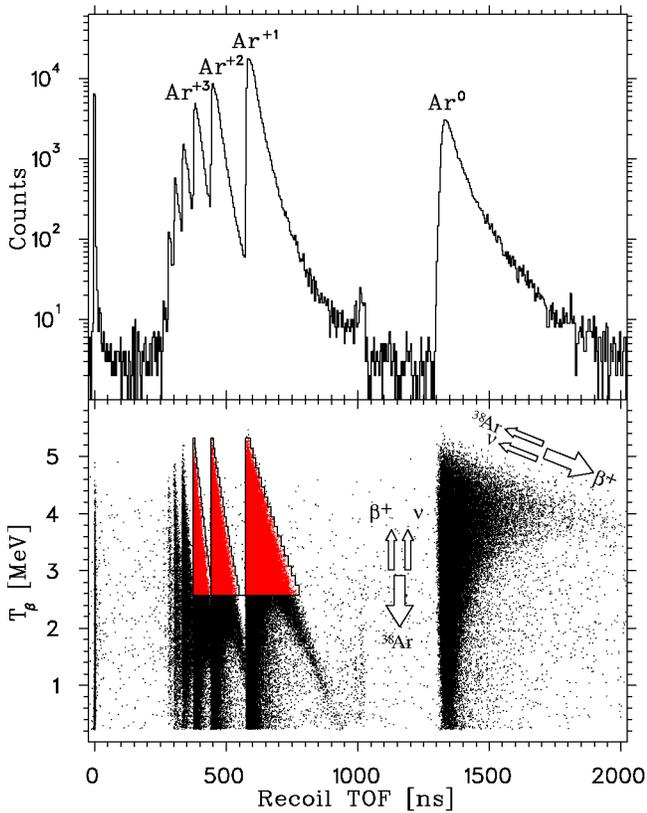
FIG. 2 (color online). Bottom: Scatter plot of recoil TOF vs  $T_{\beta}$  with one dot shown for each of 500 000 events. The suppressed back-to-back lepton emission produces longer recoil TOF. The  $E$  field separates the Ar charge states. The analysis cuts are shown. Top: TOF projections of the 2D scatter plot. The 0.1% background at TOF  $\approx 1020$  ns is from  $\beta^+$ 's scattering off the MCP into the  $\beta$  telescope and can be rejected kinematically.
