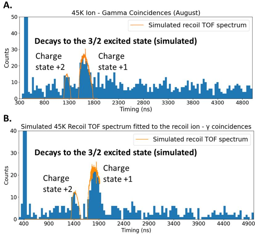
**Fig. 6.** 45K recoil ion – gamma ray coincidence spectrum for the **A.** August run and **B.** December run. The orange lines represent the TOF simulations for the decays of the recoil 45K to the  $3/2$  excited state for charge states +1 and +2.
