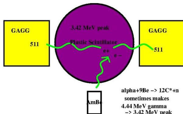
**Fig. 3.** Schematic for the AmBe experiment showing the decay process and the GAGG detectors placed at the sides of the plastic detector. This figure lacks the polyethylene block between the plastic scintillator and the AmBe source.
