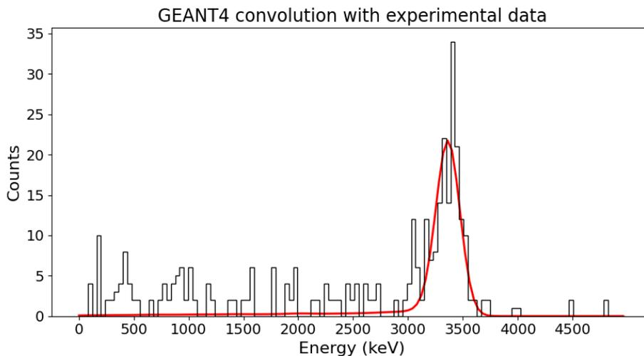
**Fig. 5.** The energy spectrum for the plastic detector shows the double escape peak at 3.42 MeV. The red solid line represents the GEANT4 simulation convolved with a Gaussian function.
