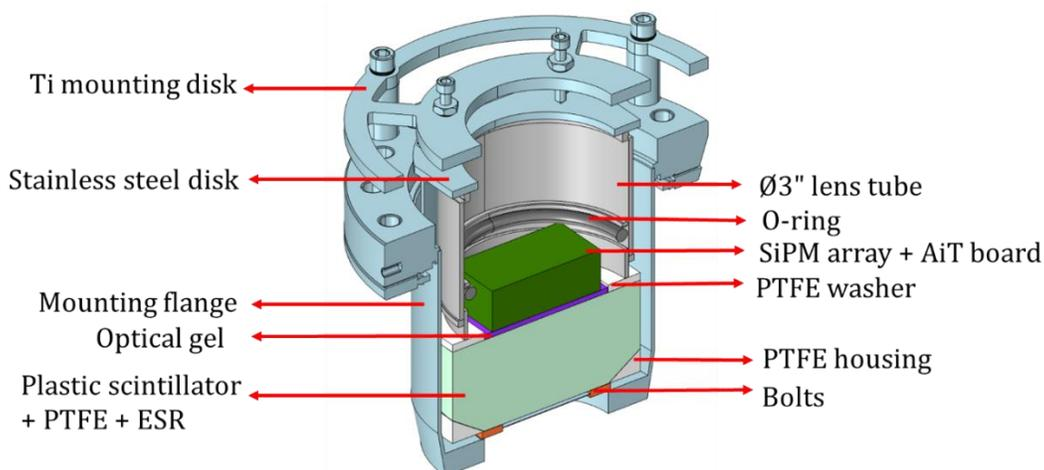
**Fig. 2.** The new plastic scintillator detector assembly with the housing design inside the mounting flange. The plastic scintillator is wrapped with  $\sim 10$  layers of PTFE and one layer of ESR. This figure lacks another layer of Teflon sheet and ESR on top of the PTFE washer.
