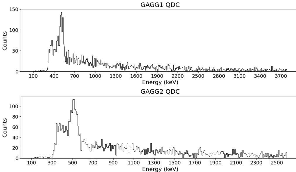
**Fig. 4.** The energy spectrum for both GAGG detectors after implementing the triple gamma-ray timing coincidence. The spectra clearly show the annihilation peaks around 511 keV.
