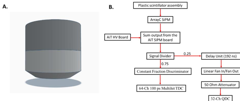
**Fig. 1.** Plastic scintillation detector setup. **A.** 3D model of the plastic scintillator attached to the light guide. **B.** Schematic diagram of the data acquisition system for the detector.
