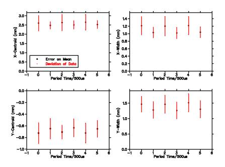
Figure 18: Cloud shape measurements for the sine-boost waveform.
