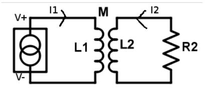
Figure 4: The equivalent circuit used to model the main coils and a coupled conductor. The main coils, of self-inductance  $L_1$ , are driven by a current generator. The coupled conductor has a self-inductance of  $L_2$  and a resistance of  $R_2$ . The mutual inductance between the main coils and the coupled conductor is M. The current in the main coils and the coupled conductor is  $i_1(t)$  and  $i_2(t)$  respectively, with the directions as indicated.
