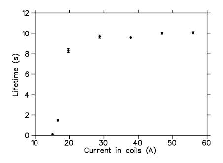
Figure 14: Plot of the lifetime of the trap versus the current in the main coils (and therefore the magnetic field strength) for a DC trap.
