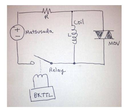
Figure 22: Sketch of circuit for fast shut-off of current in coils.
