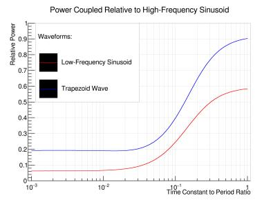
Figure 5: Plot of the ratio of the power coupled by a given waveform to the power coupled by the high-frequency sinusoid as a function of the parameter  $\tau/2T_0$ . For the pellicle mirror mount,  $\tau/2T_0 \approx 0.0215$ . At this value on the x-axis, the low-frequency sinusoid couples 12.8 times less power than the high-frequency sinusoid and 2.5 times less power than the trapezoid wave.
