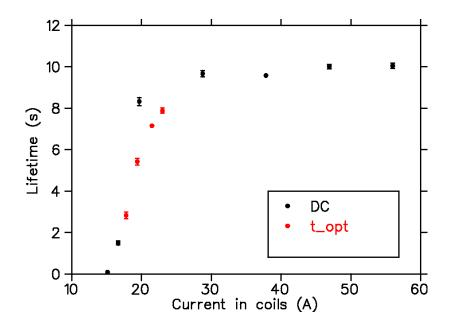
Figure 19: A plot of the lifetime versus average current. In black are the DC measurements and in red are the equivalent average currents calculated for the different optical pumping time measurements.
