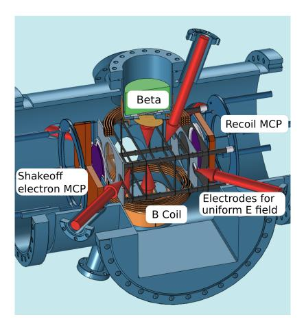
Figure 2: Diagram of the TRINAT MOT chamber.
