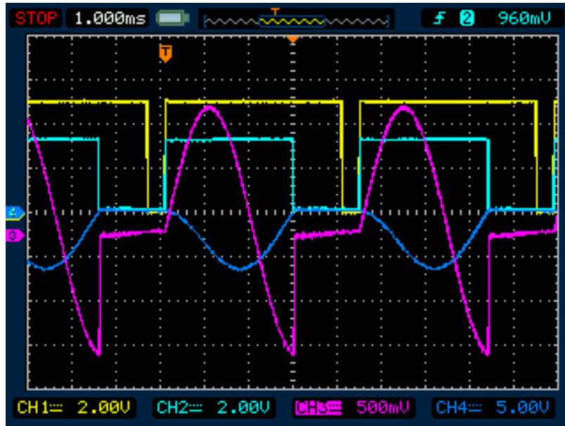
Figure 6: The blue waveform is a measure of the (inverted) current output of the Matsusadas. The pink waveform is the voltage input to the Matsusadas. The cyan waveform is a TTL logic signal which triggers each pink sinusoid and amplitude modulates the same.
