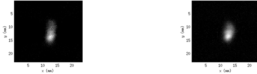
(a) AC MOT at 144.7 MHz 5% power at 100 ms exposure, sum of 630 images (b) AC MOT at 144.7 MHz 10% power at 200 ms exposure, sum of 70 images
