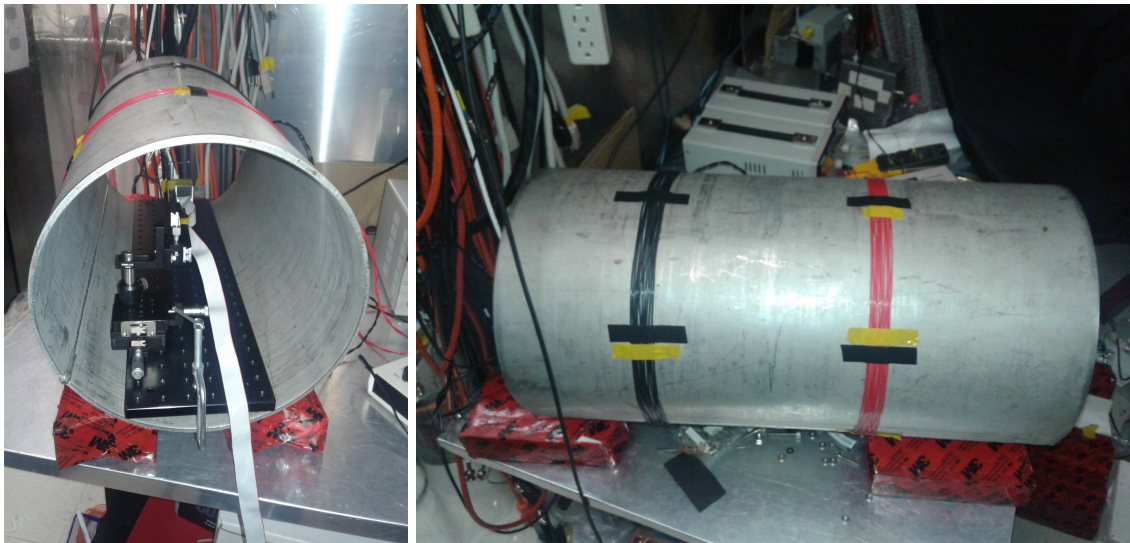
Figure 2. a) Outside view of simulation. b) Side view of simulation with black and red near-Helmholtz coils.
