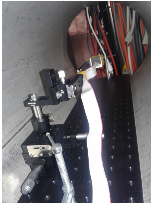
Figure 3. Inside view of simulation; x-axis is horizontal, z-axis is vertical, and y-axis is going into cylinder.
