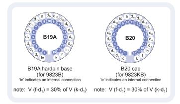
Our range of B19A sockets is available to suit the hardpin base. Our range of B20 sockets is available to suit the B20 cap. Both socket ranges include versions with or without a mounting flange, and versions with contacts for mounting directly onto printed circuit boards.
