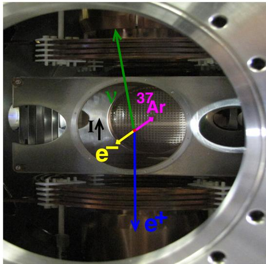
**Figure 7.** The apparatus of figure 1, illustrating the measurement of nuclear recoil,  $\beta^+$ , and shakeoff electron. Q2
